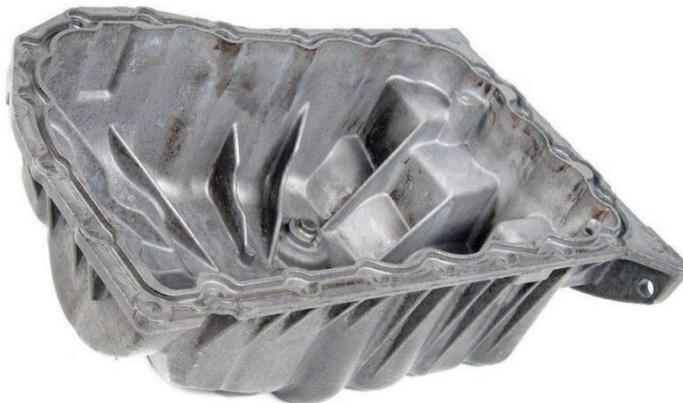
**Figura 14:** Cárter do motor
